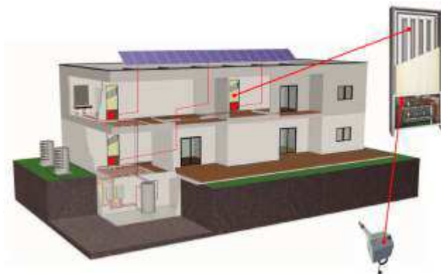
Example for hot water wall-integrated storage, copyright: Pink GmbH
